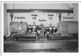
Fig.5. Mechanical diagnostic test bed.
