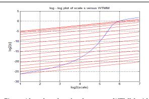
Figure 4.log - log plot of scale s versus WTMM with tangent line
